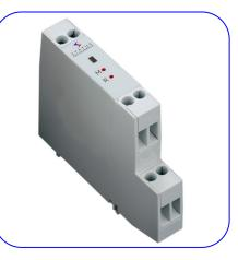
The SEM213/P is a cost effective "smart" DIN rail mount transmitter that accepts resistance temperature sensors and converts sensor output over a configured range to a standard industrial (4 to 20) mA transmission signal.
