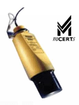
The MSP900SH/FH is a sealed 4-20mA loop powered level transmitter specifically designed for use in waste water and effluent treatment plant on aqueous applications. Certified Intrinsically Safe for use in Zone 0 areas, the rugged UPVC transmitter is factory fitted with up to 50m / 165ft of two core cable for simple low cost installation in sumps, wet-wells and over open channel flow structures.
