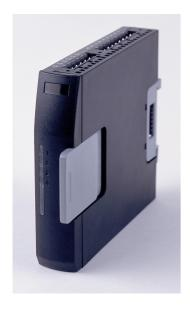
Each four Loop Module is an independent PID controller with 4 input and 6 outputs. Up to a max of eight Loop Modules can be connected to a single Bus Module making it possible to have up to 32 loops of independent control. Mixed installations of Single, Three and Four Loop Modules are possible. Each Loop Module can be removed and replaced (Hot Swapped) whilst the process is running.
