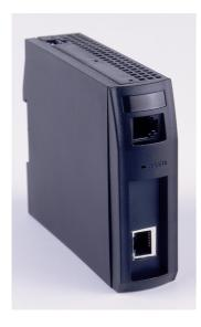
The Ethernet/IP Bus Module is part of the MLC 9000+ DIN-Rail mounting multiple loop PID control system. The Bus Module is the supervisor in the MLC 9000+ system and manages the communication with up to 8 single or multiple Loop Modules and the Ethernet/IP network. Systems larger than 32 loops can be built using multiple Bus Modules, within the limitations of your Ethernet/IP system.
