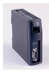
The PROFIBUS Bus Module is part of the MLC 9000+ DIN-Rail mounting multiple loop PID control system. The Bus Module is the supervisor in the MLC 9000+ system and manages the communication with up to 8 single or multiple Loop Modules and the PROFIBUS network. Systems larger than 32 loops can be built using multiple Bus Modules, within the limitations of your PROFIBUS system.
