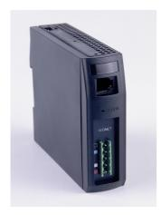
The CANopen Bus Communications Module (BCM) is part of the MLC 9000+ DIN-Rail mounting PID control system. The BCM handles communication between up to 8 single or multi loop controller modules and the CANopen network. Systems larger than 32 loops can be built using multiple BCMs, within the limitations of your CANopen system.
