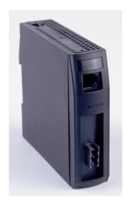
The MODBUS Bus Module is part of the MLC 9000+ DIN-Rail mounted multiple loop PID control system. The Bus Module is the supervisor in the MLC 9000+ system and manages the communication with up to 8 single or multiple Loop Modules and the MODBUS RTU network. Systems larger than 32 loops can be built using multiple Bus Modules, within the limitations of your MODBUS RTU system.
