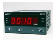
The West 8010 is a 1/8 DIN microprocessor based digital indicator. Available with red or green displays. One latchable relay is fitted as standard, plug-in modules allow two more alarm relays, PV retransmission or transmitter PSU.
