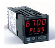
The West 6700+ is a programmable safety cut out with optional outputs for annunciators and alarms. A latched relay cuts power to your process if safe values are exceeded. The unit must be reset before the process can continue. It has the improved Plus Series hardware and user interface for optimal ease of use.
