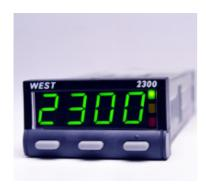
The West 2300 is available as an indicator or controller. Small size does not come at the expense of features, they have large 10mm high displays, 2 amp relays and full 3-wire PT100 inputs. The controller features our hands-free Easy Tune PID algorithm
