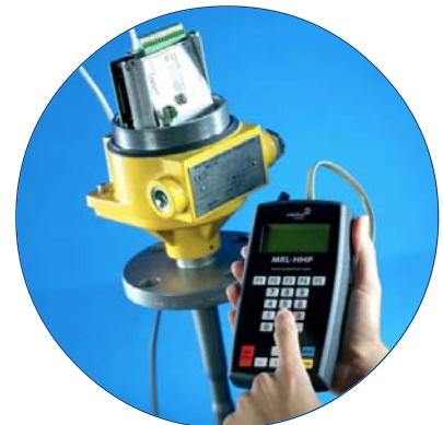
HHP connected to transmitter
