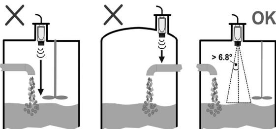
Obstructions in the tank or well may generate echoes which can be confused with the real liquid surface echo. Obstructions within the beam angle generate strong "false-echoes"; wherever possible, the transmitter should be positioned such that false echoes are avoided.
