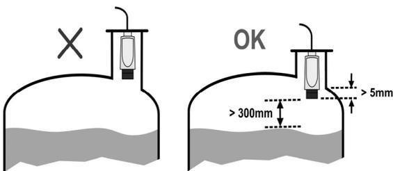
If the transmitter is mounted in a stand-off or nozzle, it is always preferable that the transmitter face be at least 5mm proud of the stand-off such that it protrudes beyond the stand-off and into the tank.
