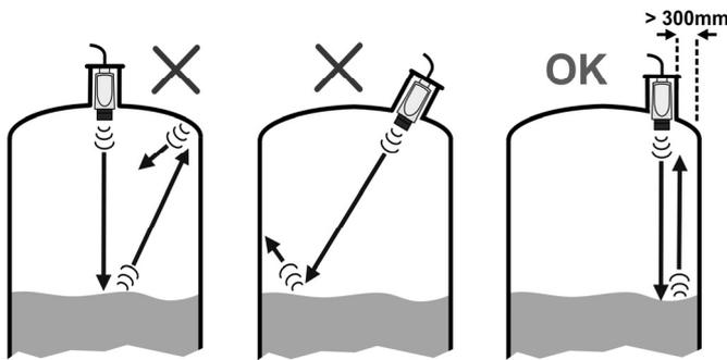
The transmitter should be mounted as near vertical as possible to ensure a good echo from the liquid surface and maximum echo size received. The beam angle (to the half power point) of the transmitter is 12 degrees inclusive.
