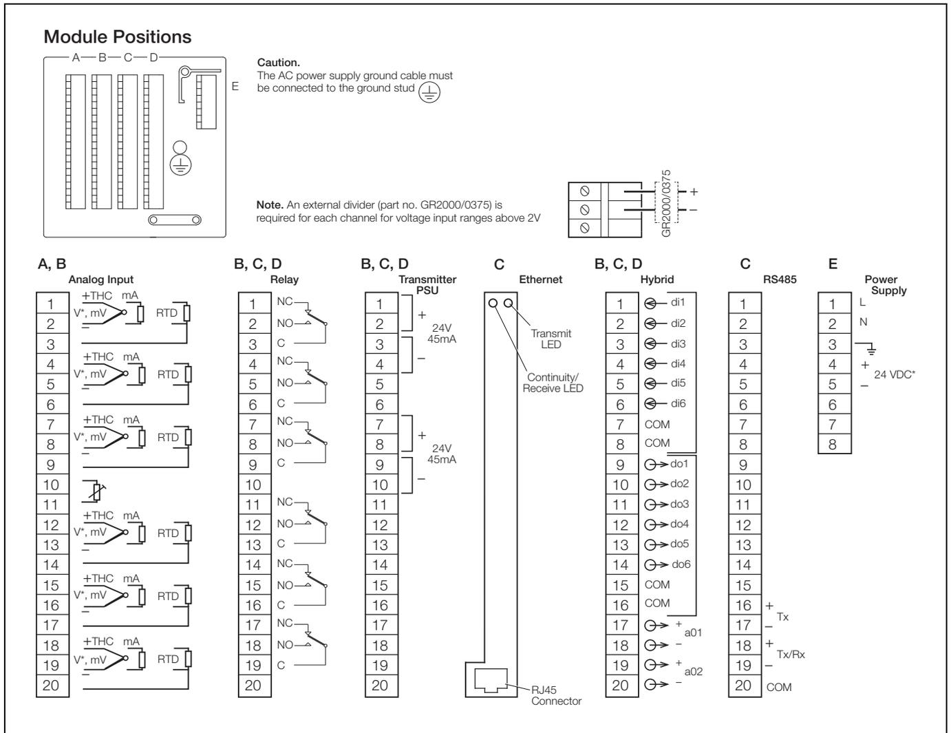
\*Note. 24 V DC instrument power supply must be specified when ordering.
